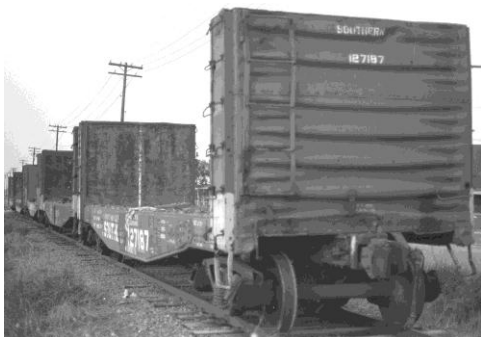
Top: 128980 at Columbus, GA on 3/15/69. Middle & Right: 127187 in Charlotte, NC storage line on 6/5/80. All photos by Larry Goolsby. Note that stenciling diagram shows "B" end lettering applied to separate plate; "A" end photos show lettering applied directly to the ribs, centered across the car's width. The white, bulkhead centerline stripe clearly shows in each photo.
