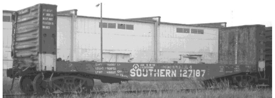
Top: 128980 at Columbus, GA on 3/15/69. Middle & Right: 127187 in Charlotte, NC storage line on 6/5/80. All photos by Larry Goolsby. Note that stenciling diagram shows "B" end lettering applied to separate plate; "A" end photos show lettering applied directly to the ribs, centered across the car's width. The white, bulkhead centerline stripe clearly shows in each photo.
